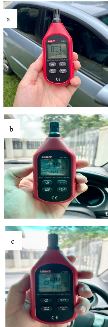
Fig. 12: (a) measured ambient air temperature, (b) measuring initial Car's interior temperature and (c) measuring average Car's interior temperature
