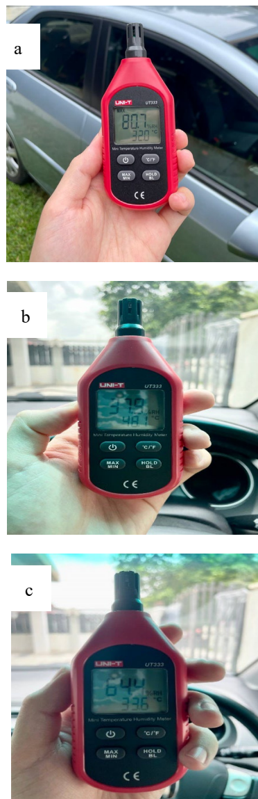
Fig. 12: (a) measured ambient air temperature, (b) measuring initial Car's interior temperature and (c) measuring average Car's interior temperature
