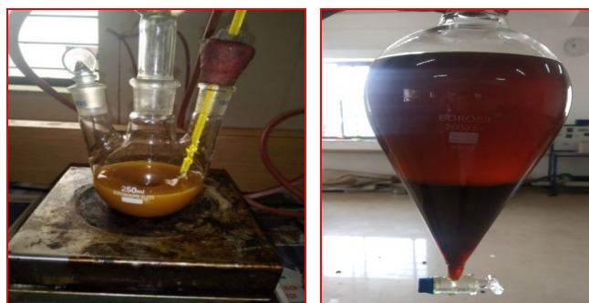
Fig. 2: Esterification set-up (left side) and gravity separation (right side)
