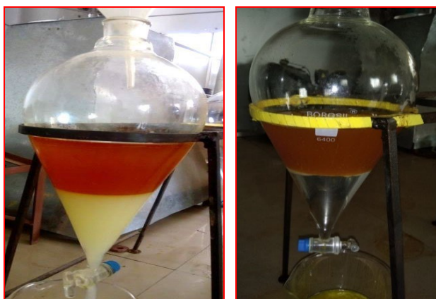
Fig. 3: Water washing first stage (left side) and final stage (right side).
