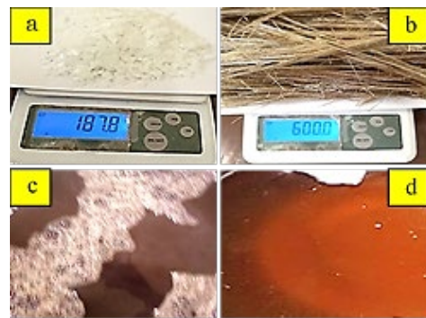
Fig. 2: Alkali treatment of BF: a) NaOH flakes, b) measuring of BF, c) and d) removed impurities after AT
