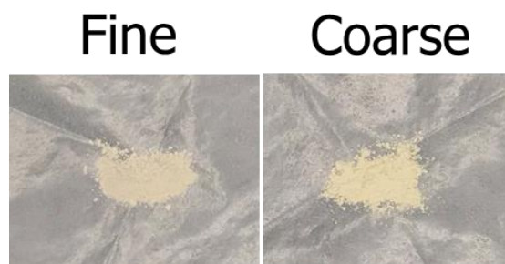
Fig. 3.7 Color of separated \text{SnO}_2 ; identical tendency with hydrothermal treatment.
