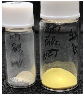
Fig. 3.4 Color of separated \text{SnO}_2 synthesized by hydrothermal treatment: white (left) is fine- \text{SnO}_2 and yellow (right) is coarse- \text{SnO}_2 .
