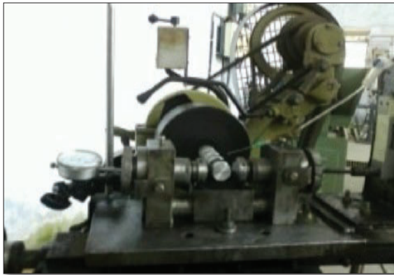
Fig. 3: Experimental setup of burnishing tool.
