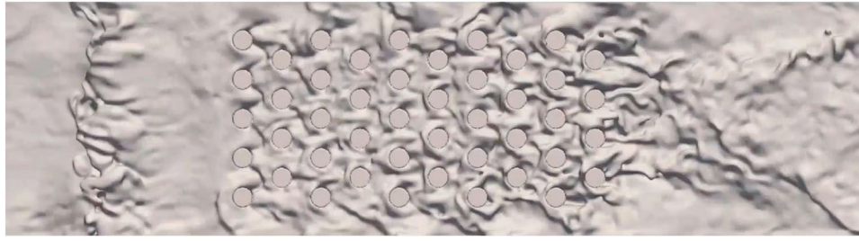
Figure 14. Top view of simulation result of tsunami against tide protection forest.
