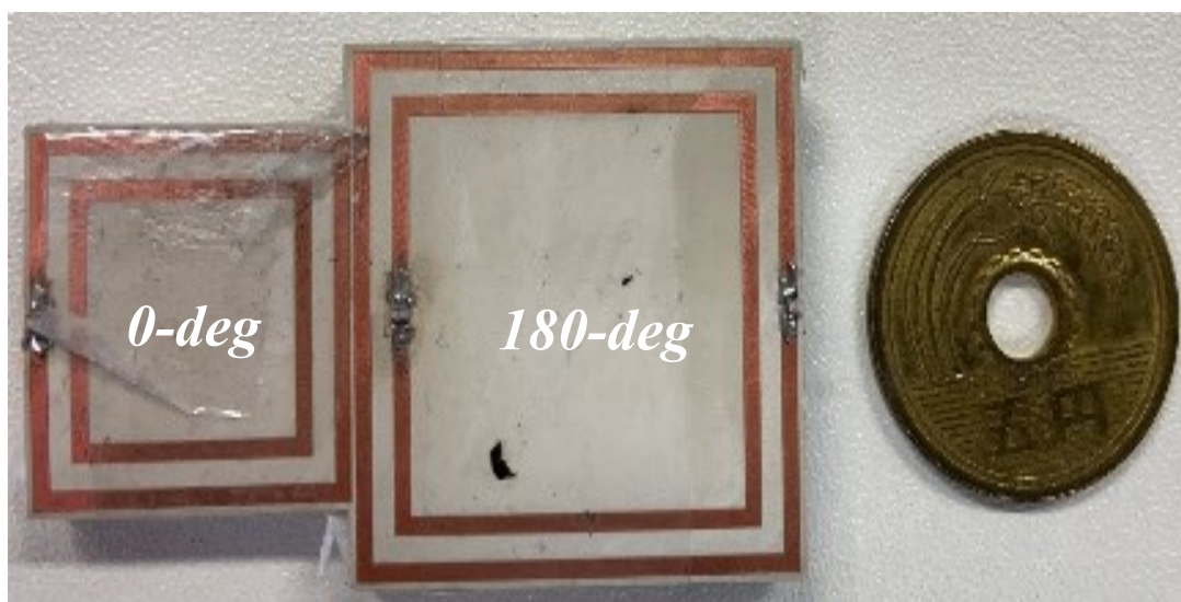
Fig. 21 Proposed metasurface. “0-deg” stands for the 0-degree Metamaterial, and “180-deg” stands for the 180-degree Metamaterial.
