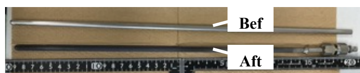
Figure 6.5. Appearance changes of the Inconel 600 tube before and after the experiment.
