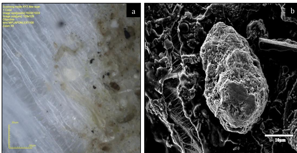
Figure II. Particle matter accumulation on Elaeagnus pungens (A) Morphological structure of the leaf surface (3D Laser Measuring Microscope -100x) (b) Scanning Electron Microscope image of particulate matter on Elaeagnus pungens filters after filtration.
