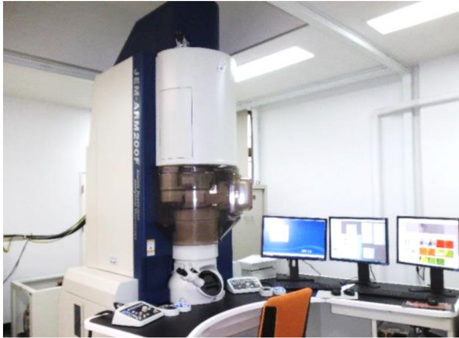
Figure 3.16 Overview of JEM-ARM 200FC with EDS Analysis
