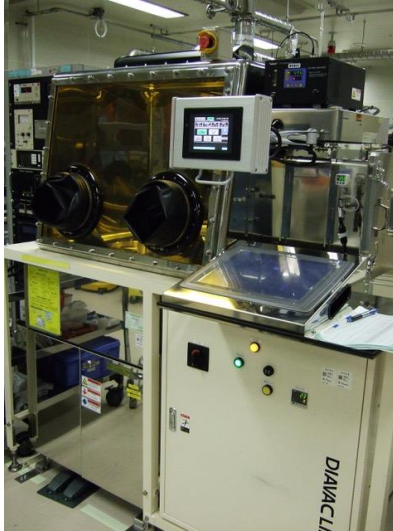
Figure 33: ALD equipment with a glove box.
