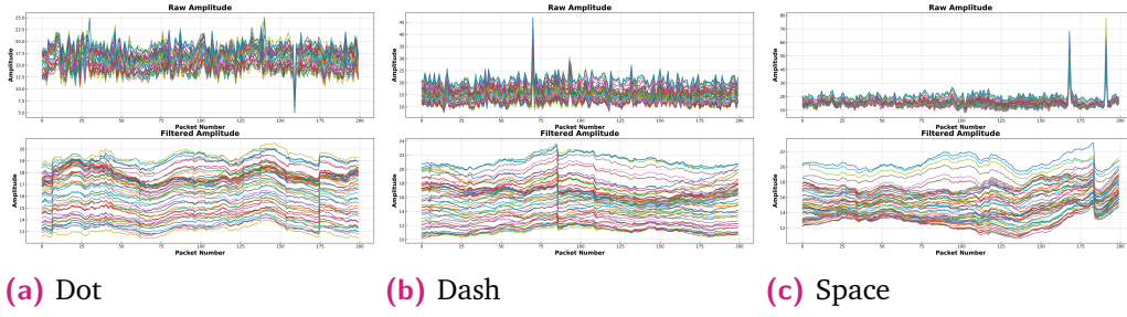
Figure 5.3: Raw and Filtered Amplitudes of Three Symbols across All Subcarriers in 1 st Link
