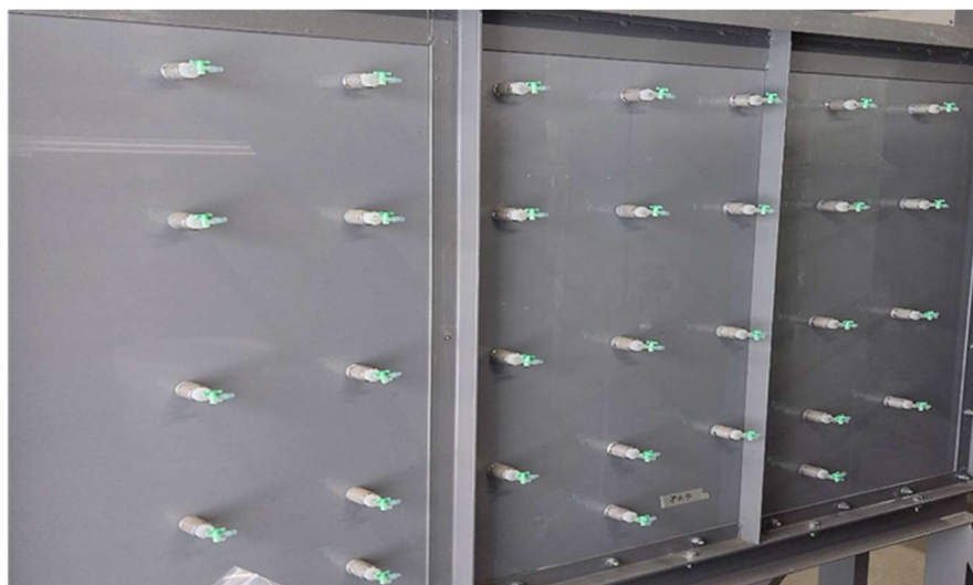
Figure 3-4. Lysimeter Rear view showing gas sampling ports.
