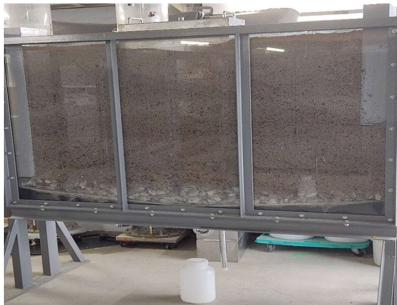
Figure 3-3. Filled Lysimeter Front View- 2 Vents
