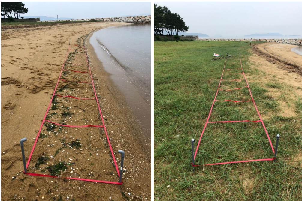
Fig. 4.1 Marine debris sampling on the foreshore (left) and backshore (right)
