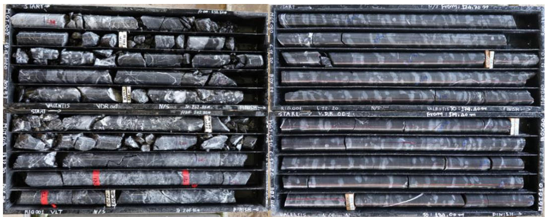
Figure 4. 5 Nalou formation dolomite (DOL) and discovery formation calcareous shales (CSH)
