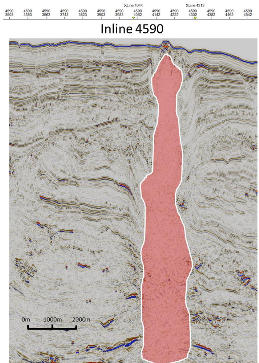
Figure 4.6 The seismic profile of inline 2,4590 was used to train the CNN for gas chimney identification. Two training classes were used, and slump units were highlighted on this profile.
