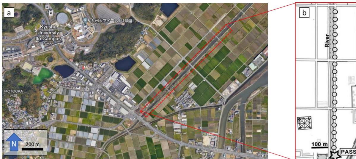
Figure 3.5 (a) the satellite image for the Riverbank field experiment near Kyushu University, (b) the profile of the survey area showing the locations of the PASS (star) and the 900 m array of geophones (Tsuji et al., 2022).
