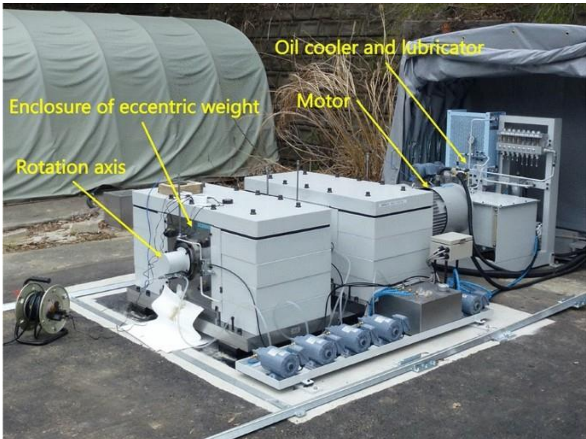
Figure 1.4 ACROSS source used in a previous study. Eccentric weights rotate around a horizontal axis to produce a sinusoidal signal (Suzuki et al., 2021; Yamaoka et al., 2014).
