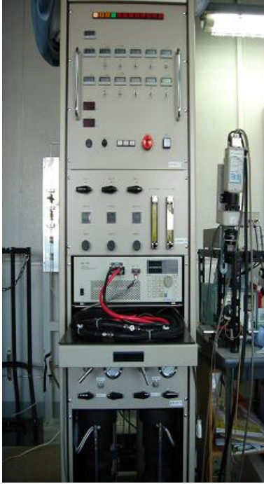
(a) The PEFC performance test apparatus.
