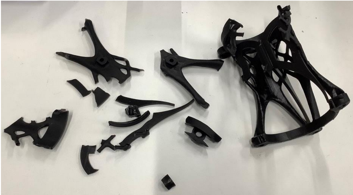
Fig. 3.1 Components manufactured by SLA 3D printer that have sustained unexpected damage.
