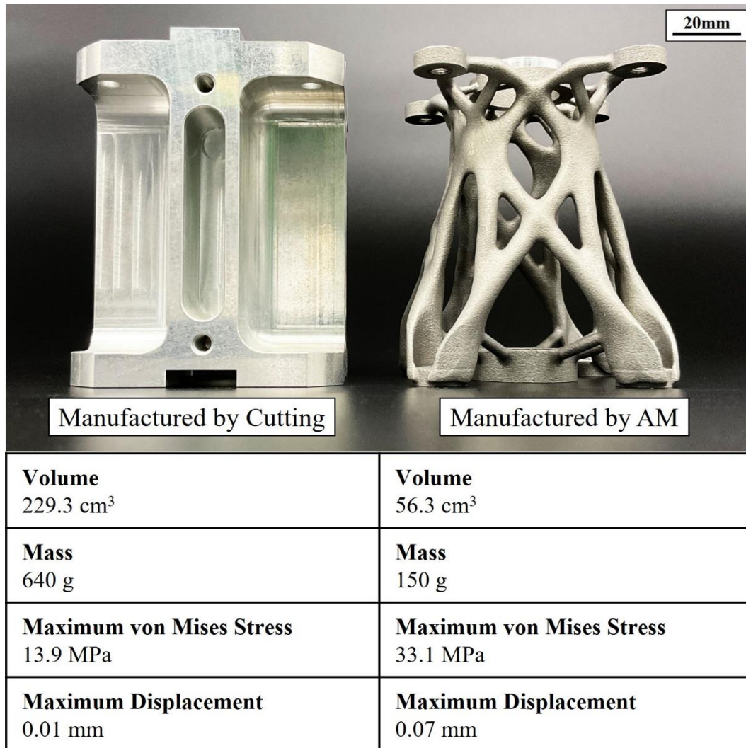
Fig. 2.6 Comparison of two types of “Arm Blocks”.
