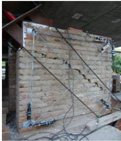
Figure 4.3: Diagonal compression test on unreinforced specimen
