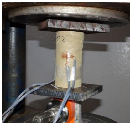
Figure 3.6: Uniaxial compression test on mortar cylinders
