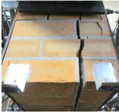
Figure 7.6: Cracks observed at the tip of the embedded anchor
