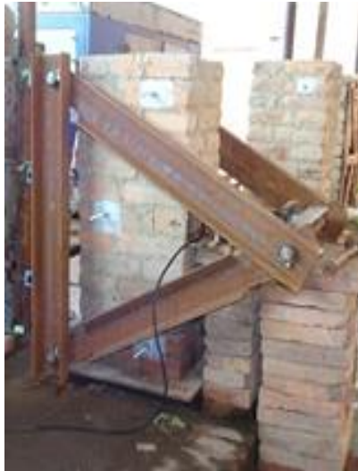
Figure 4.6: Bending test on unreinforced prism
