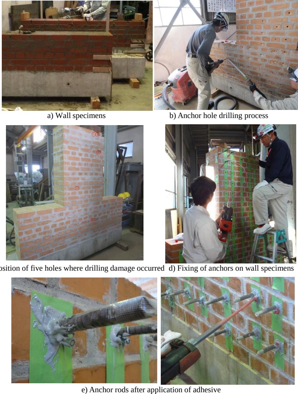
Figure 7.3: Drilling of holes and fixing of anchors on wall specimens
