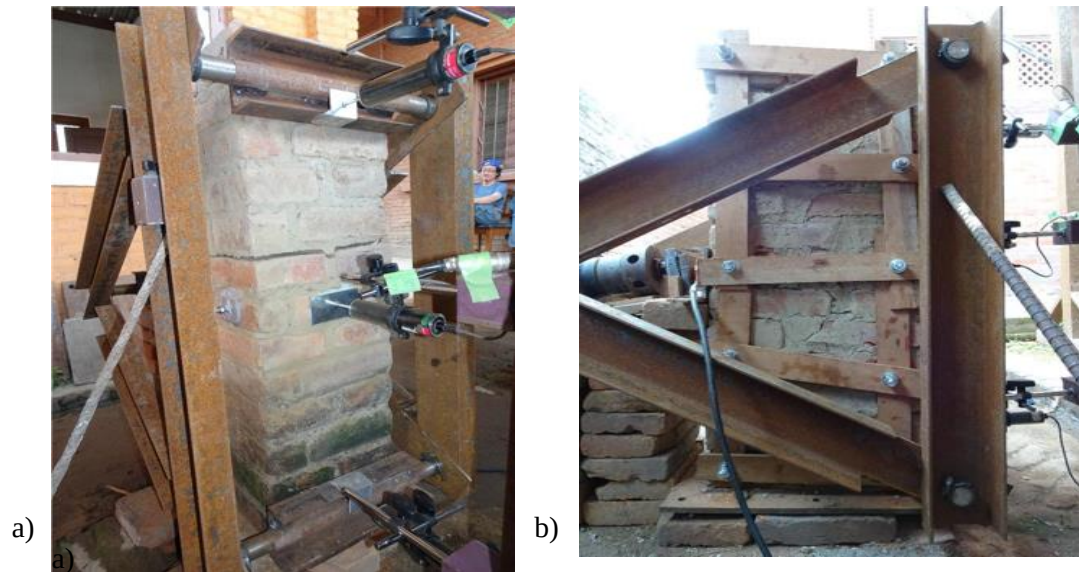
Figure 4.13: a) Crack pattern in specimen B5U1; b) Crack pattern in specimen B1L1
