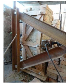
Figure 5.1c): Diagonal brace reinforced specimen
