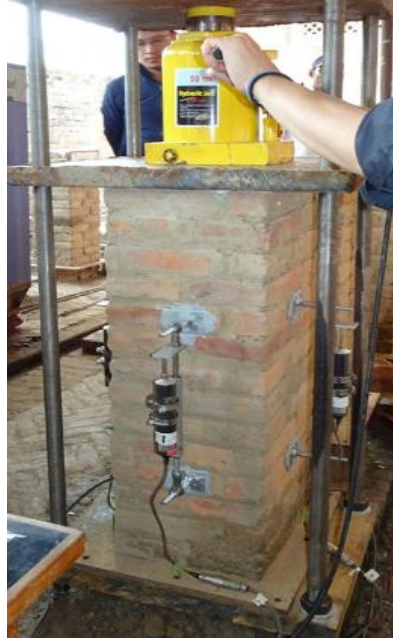
Figure 3.7: Uniaxial compression test on masonry prism
