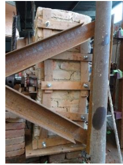
Figure 5.1b): Ladder type reinforced specimen
