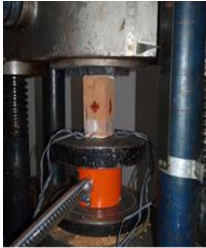
Figure 3.5: Uniaxial compression test on unit bricks
