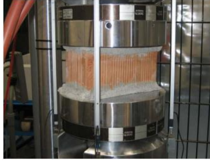
Figure 2.8: Compression test on a brick specimen (Bergami, 2007)
