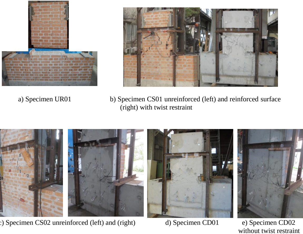
Figure 7.13: Cracks and failure mode of specimens
