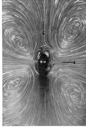
Fig. 14 Circulatory streaming around an elliptic cylinder at r_0\sqrt{\omega/\nu}=8.34 . r_0=0.206 cm, f=60.6 Hz, s=0.0312 cm, \nu=0.232 cm 2 /s, r_0\sqrt{\omega/\nu}=8.34 , s/r_0=0.151 , t_e=30 s. Glass micro-particles were added to serve as tracers.
