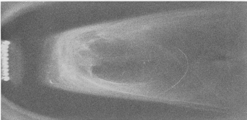
Photo 11 Same as Photo 10, but a tracer generating wire is located just upstream of the same test body: U = 2.36 cm/s, R_s = 18.3 , R_g = 264 .
