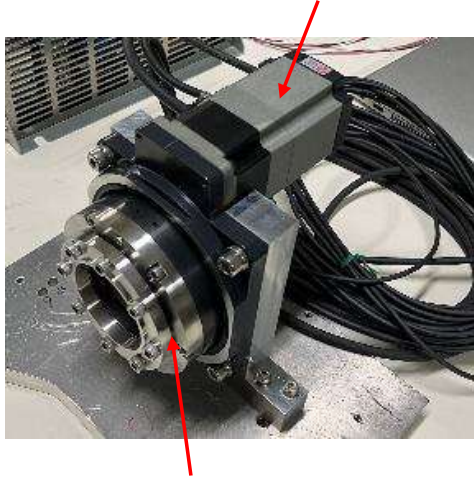
Vacuum rotary feedthrough (hollow shaft, magnetic coupled)
