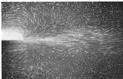
Photo. 9. Like Photo. 8, but R_1 is about twice that for Photo. 8; U_1=0.347 cm/s, U_2=1.35 cm/s, a=0.531 cm/s 2 , t=5.72 s, d=1.50 cm, t_e=2 s, R_1=59.1 , R_2=229 , \tau=2.24 \times 10^{-2} and \alpha=2.31 \times 10^4 .
