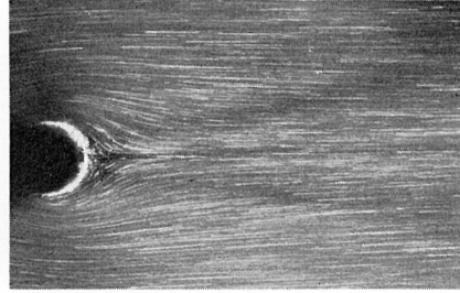
(b) Flow around the cylinder immediately after the onset of acceleration; t=3.80 s and \tau=3.31 \times 10^{-2} .
