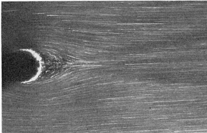
(c) Growth of the new twin vortices; t=6.47 s and \tau=5.63 \times 10^{-2} .
