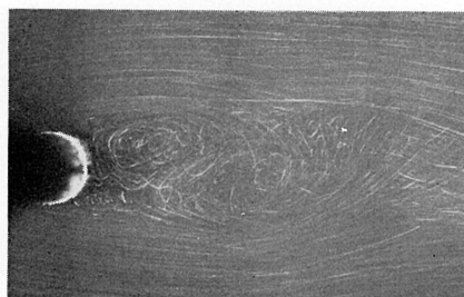
(d) Final stage of the flow at R_2 = 111 ; t = 11.5 s and \tau = 9.78 \times 10^{-2} .
