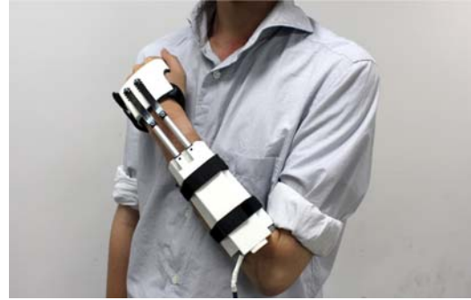
Fig. 9. An overview of the developed prototype is shown. The prototype has total weight of 509.5 g, length of 310 mm and thickness of 2.0 to 22.5 mm and can thus be worn by a user without excess effort.
