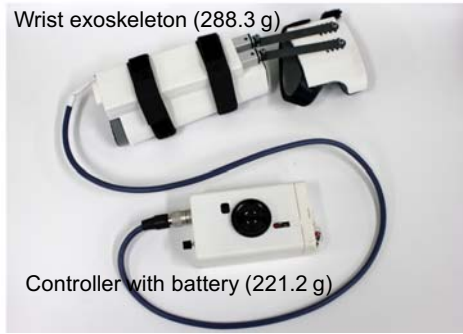
Fig. 9. An overview of the developed prototype is shown. The prototype has total weight of 509.5 g, length of 310 mm and thickness of 2.0 to 22.5 mm and can thus be worn by a user without excess effort.
