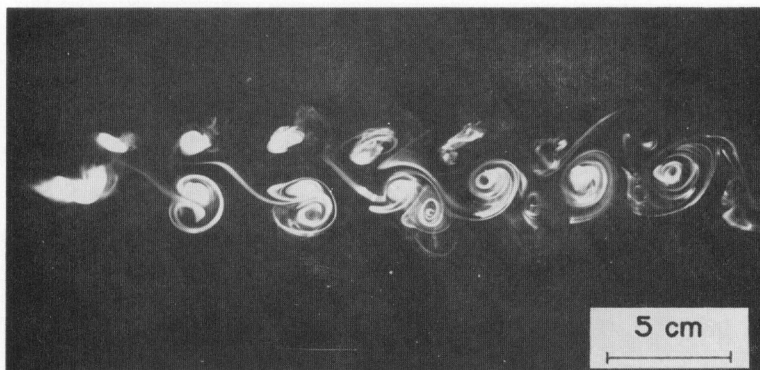
Photo. 13. Vortex wake at a large amplitude. (R=104, A/d=2.28, S_c=0.117, T_c/T_k=1.44; U_o=1.91 \text{ cm/s}, d=0.50 \text{ cm}, T_c=2.24 \text{ s})
