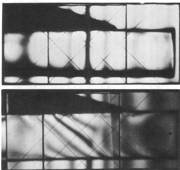
Photo 8. Occurrence of residual strains due to heat treatment
