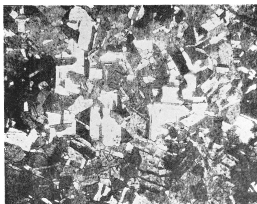
Fig. 6. Microphotograph of electrolytic copper ( \times 100 ).
