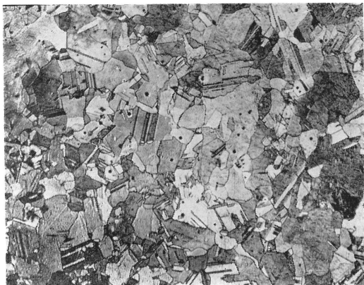
Fig. 4. Microphotograph of 70 : 30 brass ( \times 100 ).
