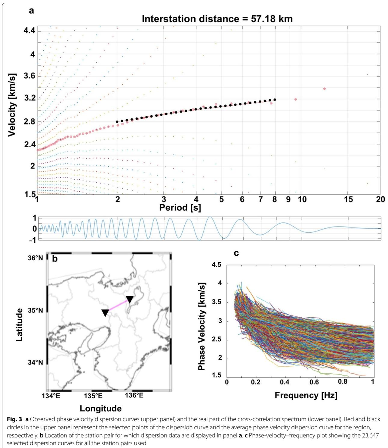
travel-time tomography at discrete frequencies. Secondly, pointwise inversion of dispersion data for 1D profiles of S-wave velocity as a function of depth at each grid point is implemented, and combining multiple 1D profiles
