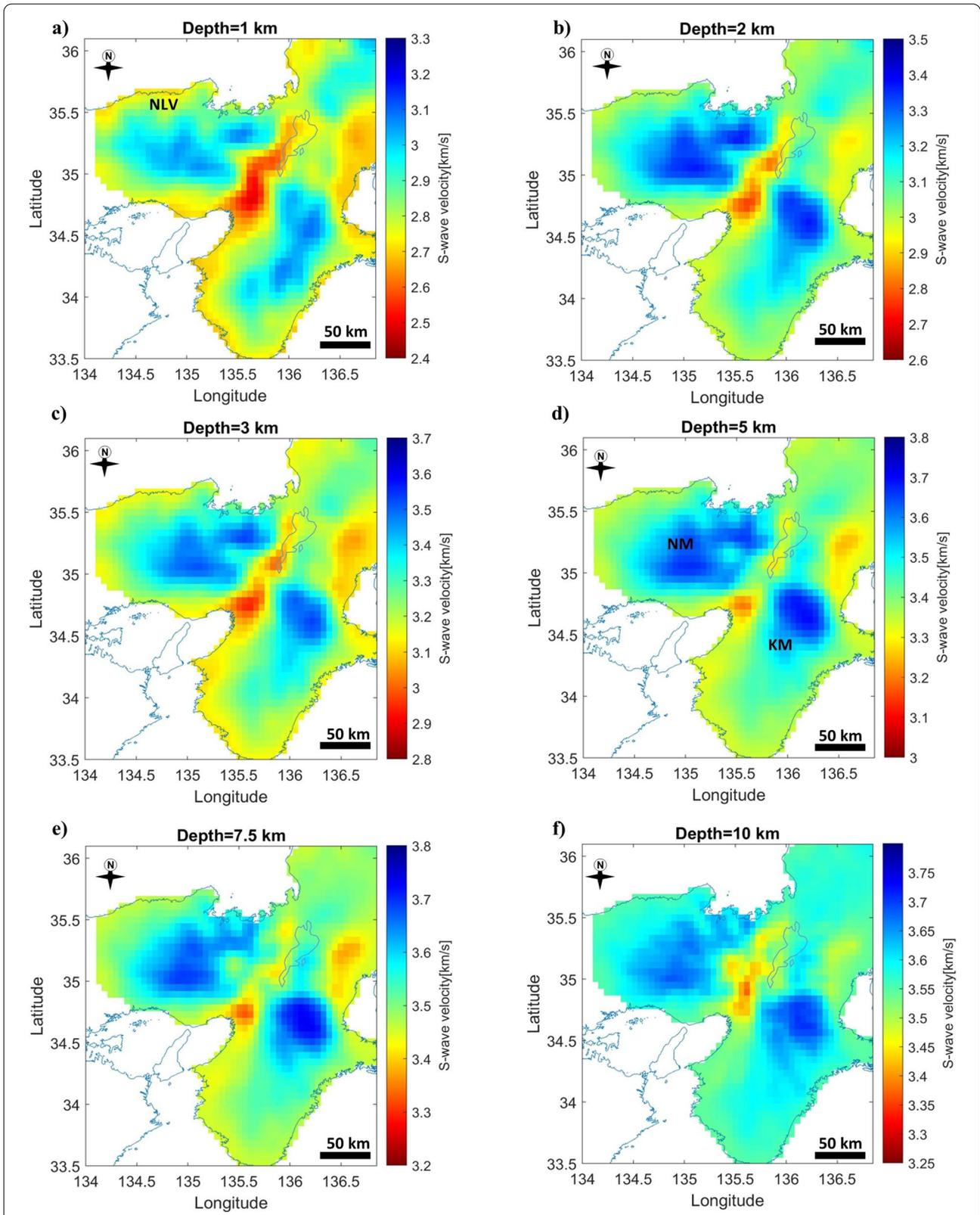
**Fig. 7** Horizontal slices of the S-wave velocity model at discrete depth levels below sea level. Depth is shown above each respective panel. **a-f** S-wave velocity models without showing the active faults (S-wave velocity models before correcting for the effects of topography are shown in Figure S4). NM and KM represent the prominent high-velocity anomalies
