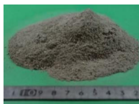
(a) Polymer modified cement powder
