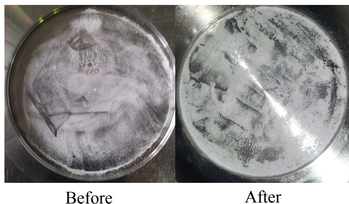
Figure 7. Photographs of the \text{SrBr}_2 sample before and after repeated cycles.
