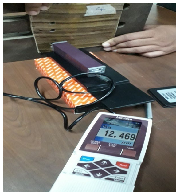
Fig. 3: Surface roughness measurement using SURFTEST SJ-210
