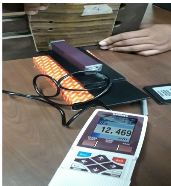
Fig. 3: Surface roughness measurement using SURFTEST SJ-210
