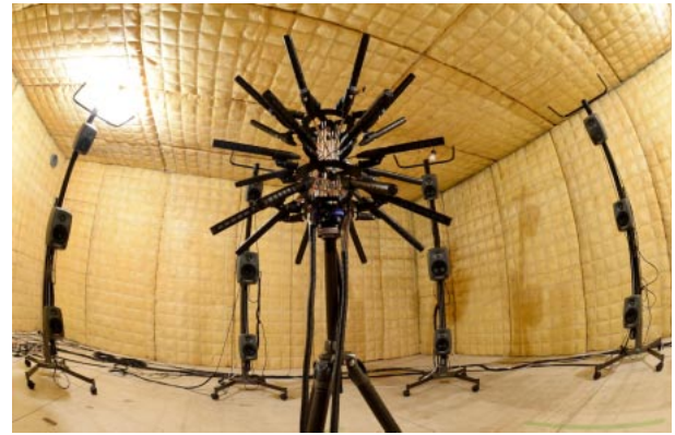
Fig. 2 Systems used in the examination, including the hedgehog shaped microphone array and the loud-speaker array called G-VRAWS.
