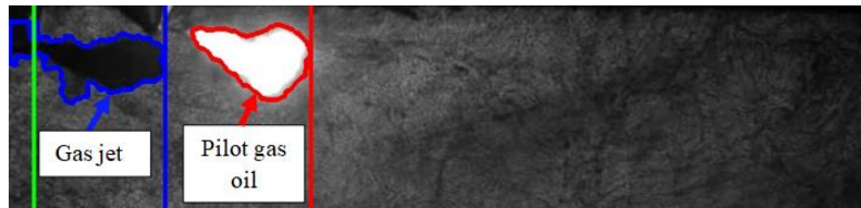
Figure 5.3 Shadowgraph processed image method
