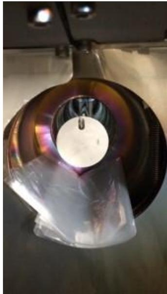
**Fig. 3.1.5 Side view from QUEST vacuum vessel. The test sample is exposed vertically to QUEST plasma using movable arm.**
