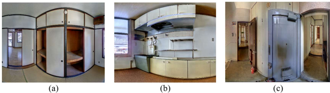
Figure 1. 3 Various forms of occlusions are present in an occupied building: (a) large wardrobe concealing one face of the wall; (b) upper cabinet resembling a short-span beam; (c) door leaning and occluding a wall surface.
