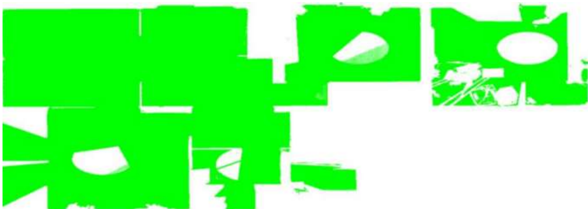
Figure 3. 7 Gaps on planar surfaces due to missing data caused by extensive occlusions.
