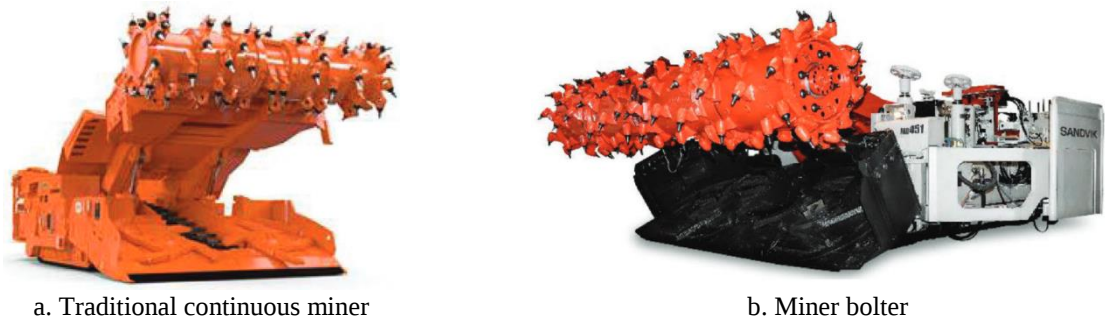
Figure 1.9. Typical techniques for gateroad development
