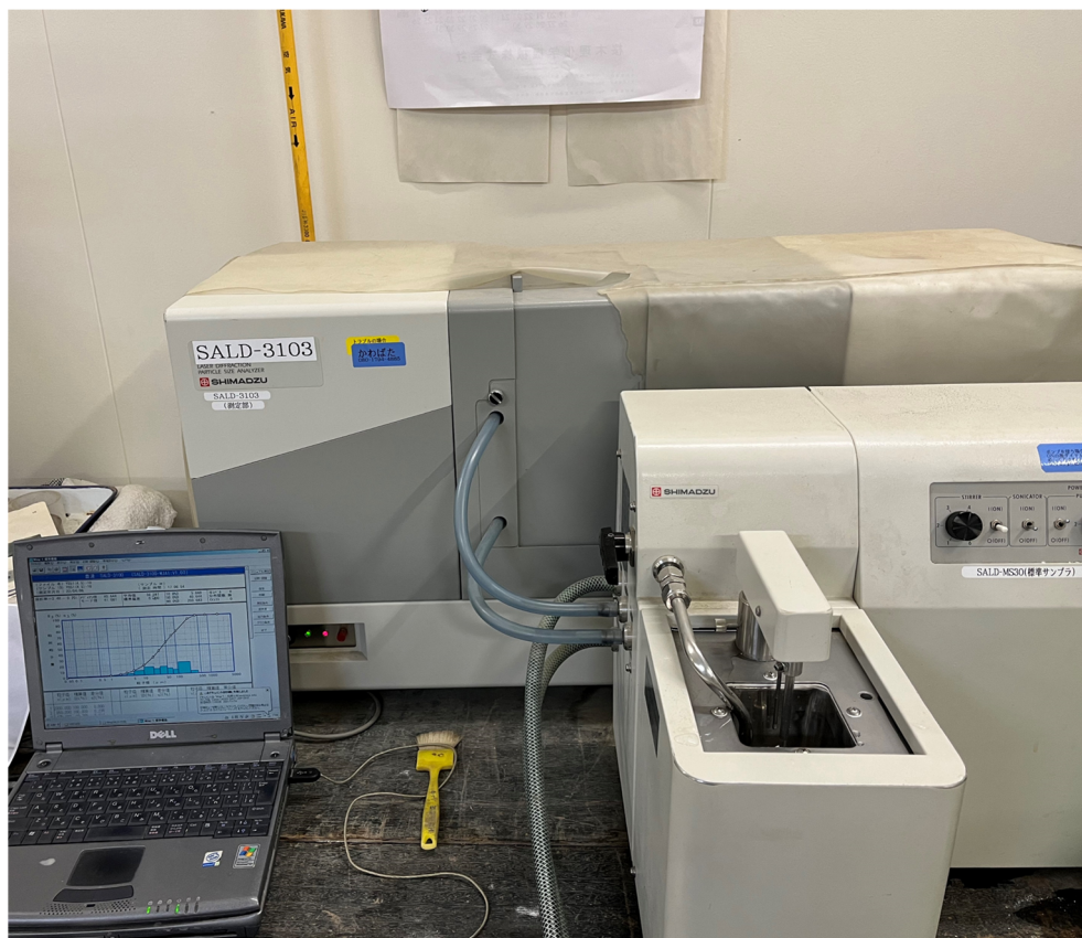
Figure 4.5 The laser diffraction particle size analyzer.
