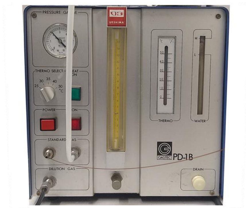
Figure S5. Photograph of the system used for sampling the gas using a fused-silica capillary from the exit port of the standard gas generator.
