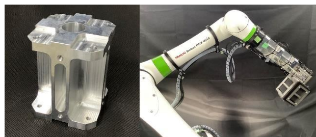
Fig. 1 "Arm Block" manufactured by cutting
