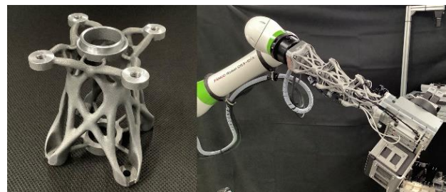
Fig. 3 "Arm Block" manufactured by AM
