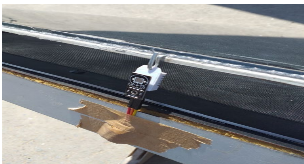
Fig. 5: Measuring the air temperature via the DHT22 sensor
