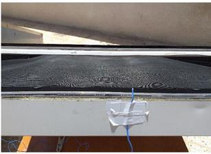
Fig. 6: Measuring the air temperature in the case of CFS
