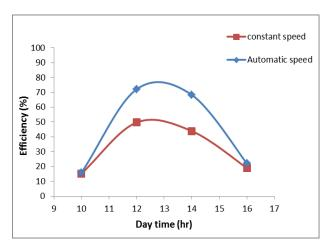
**Fig. 10:** Variation of thermal efficiency vs. local time for the SAH under the two operation modes.
