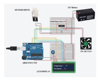
Fig. 3: Assembly circuit schematic diagram of the temperature-based fan speed control and monitoring system.
