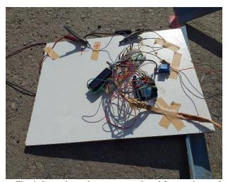
Fig. 4: Setup shows the temperature-based fan speed control and monitoring system
