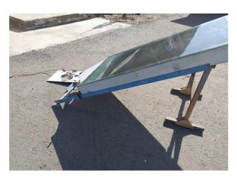
Fig. 1: The overall setup of the proposed SAH system
