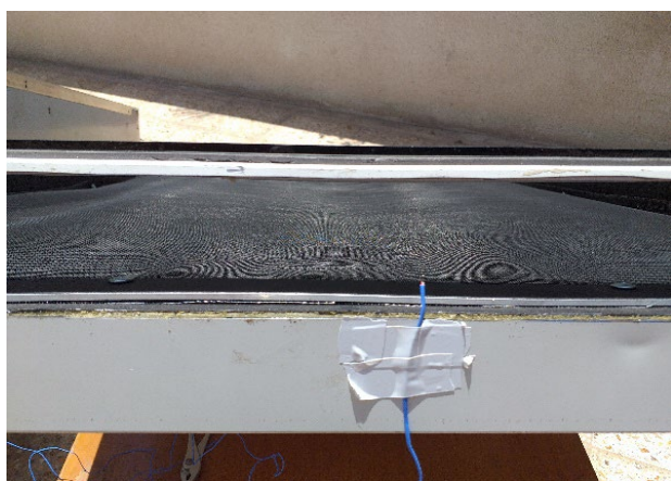
Fig. 6: Measuring the air temperature in the case of CFS
