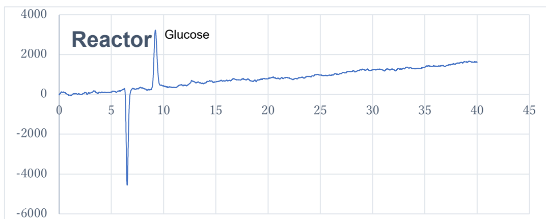
Fig. 22. HPLC chromatogram of pyrolysis of 0.1 g cellulose at 372 °C, 3.1 kPa collected from reactor after hydrolysis.
