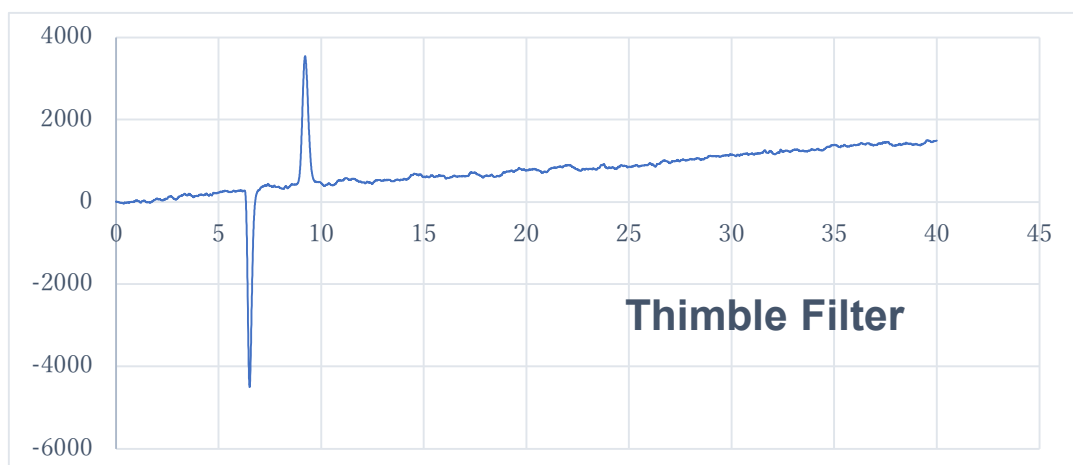
Fig. 23. HPLC chromatogram of pyrolysis of 0.1 g cellulose at 372 °C, 3.1 kPa collected from thimble filter after hydrolysis.
