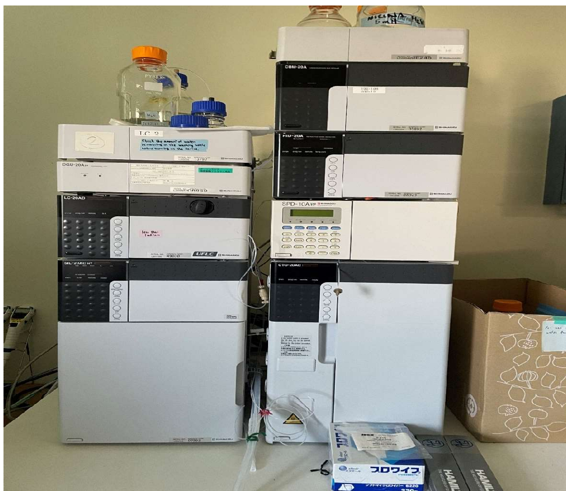
Fig. 38. High performance liquid chromatograph (HPLC) used in study.
