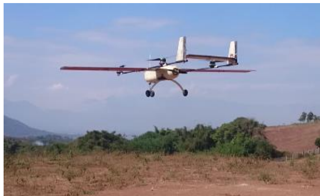
Figure 1 VTOL UAV for Aerial Surveillance Mission (Hadi, 2016)
