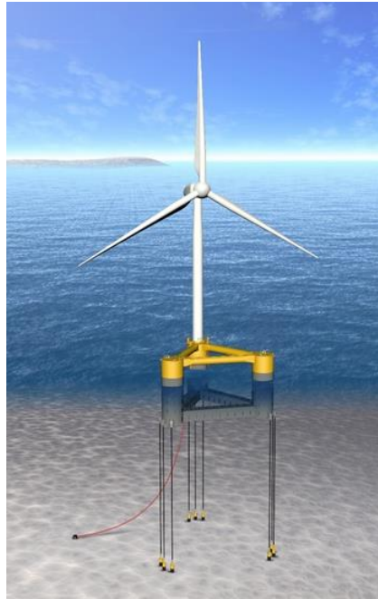
Fig. 1.1 Wind power TLP structure
