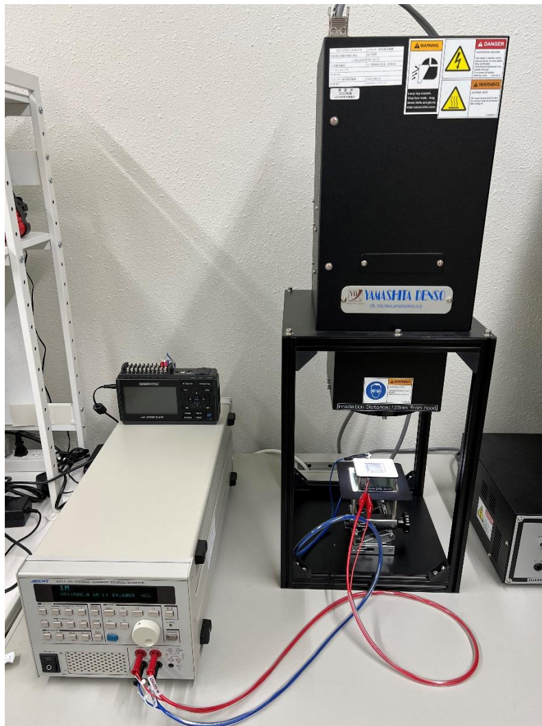
Figure 4.1. Standard-type solar simulator installed at the EES lab.
