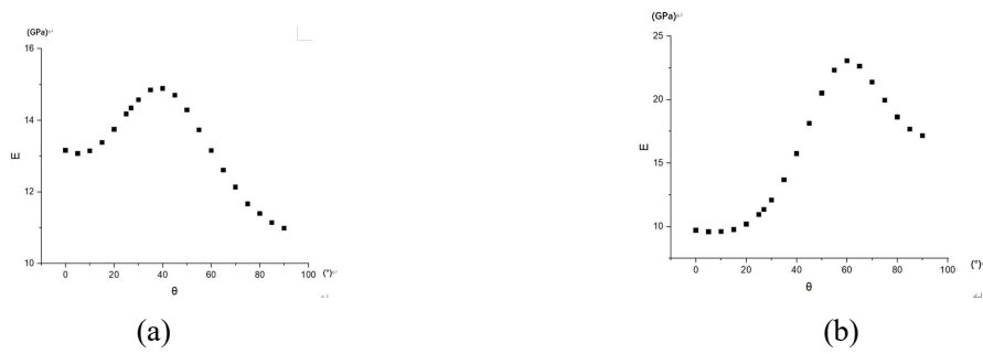
Fig.1 Variation of Young's modulus of bone as calculated from the (a)HT model, (b)PB model
