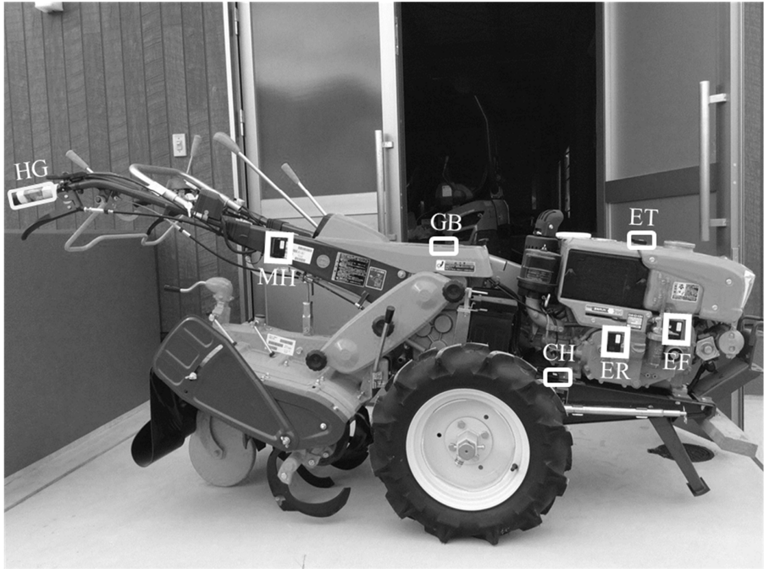
Fig. 25 Experimental hand tractor and sensor allocations
