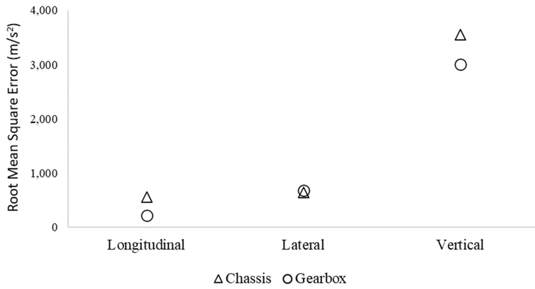
Fig. 37 A comparison of RMSE Acceleration between chassis and gearbox to the response data
