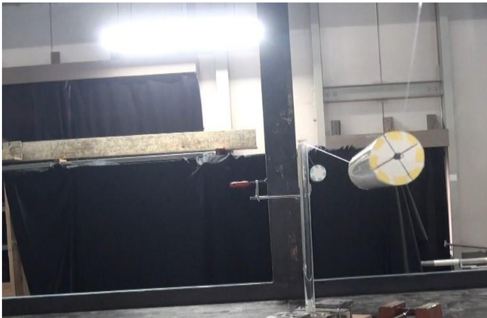
Fig 5-2. Conductor model with acrylic pipe for the wind tunnel experiment
