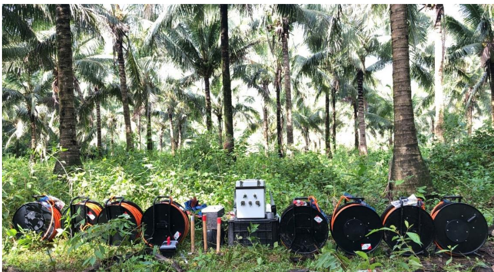
Figure 3-22. Photo of the Syscal Pro Switch 72 instrument and accessories (e.g., wire) used in the ER-IP survey.
