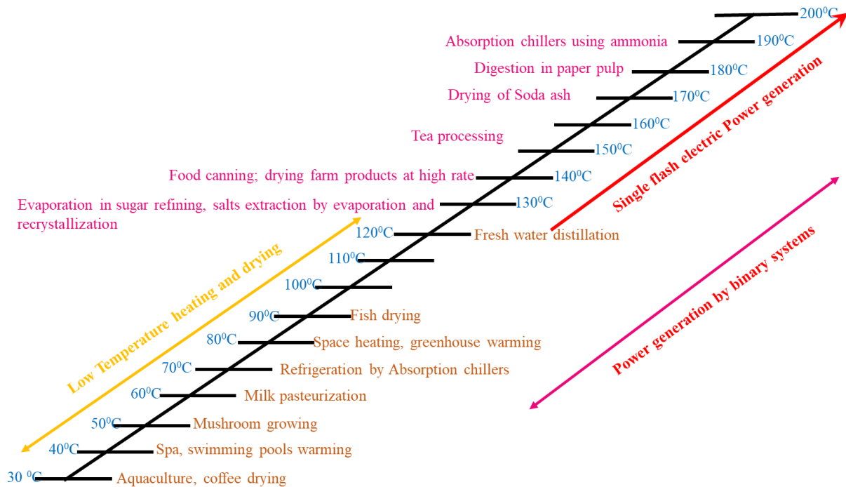
Figure 1.5 Uses of geothermal energy depending on temperature of fluid conveyed to the surface, modified from DiPippo (DiPippo, 2012)
