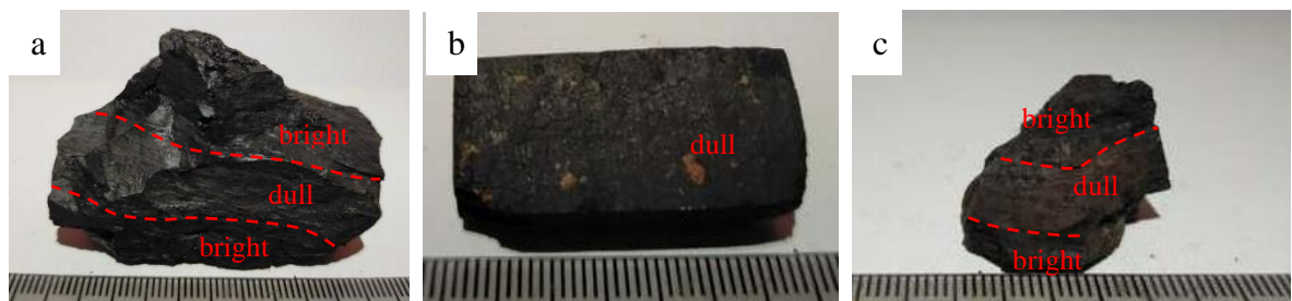
Figure 6 The lithotype of coal samples from (a) WB, (b) EB, and (c) NMTB
